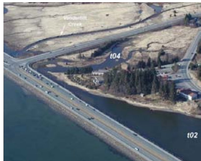
Fig 5.41 View north over Egan Drive. Vanderbilt marsh, t04, was the original estuary of Vanderbilt Creek. During Egan construction, the creek was moved to the dredged channel in distance.
